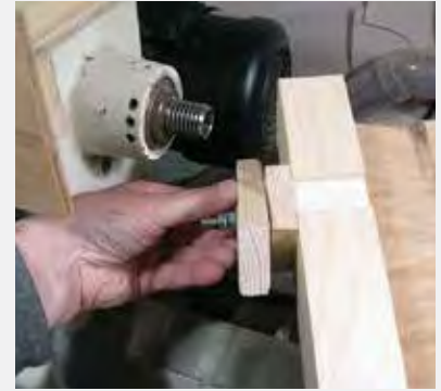
To lock the front of the headstock box in position, make a simple toggle that can be tightened under the lathe bed.
