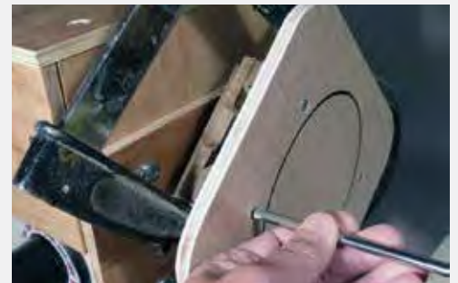
To change faceplates, clamp the runners against the slide to hold them in position while you loosen screws.
