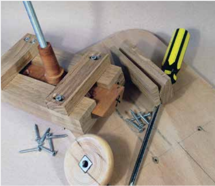
The slide mechanism moves between runners mounted on bearers that are set the cam diameter apart. The work-holding faceplate, at right, gets screwed to the runners and moves with them.
