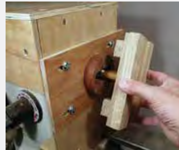
Mark a centerline squarely across the two runners, flanked by lines the cam diameter apart. Clamp or glue-tack one bearer on the line, then screw the other bearer against the cam and adjust for a firm fit.
