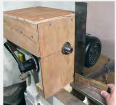
The front of the headstock box must be vertical and square to the lathe ways. Mark a horizontal line across the face of the box at center height and note how far the spindle projects, as this distance limits the thickness of the cam and bearers.
