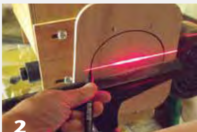
Guide the cut by shining a center-height laser line onto the faceplate. The cutting angle may not always be perfect but its position will be.
