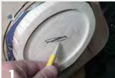
The edge of the lathe tool must cut at the lathe's center height. Deviation above or below center will create a new pathway and a confusing profile.
